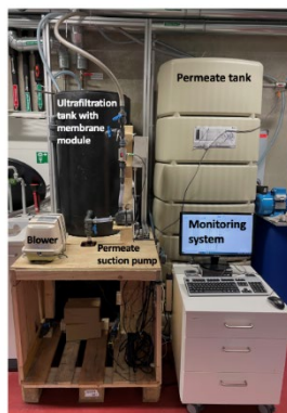
Figure 1: Ultrafiltration system with submerged Cubes® RM6 from Martin Systems GmbH setup in the laboratory of HKA University of Applied Sciences Karlsruhe (Photo Courtesy: Duc N. Dinh)
